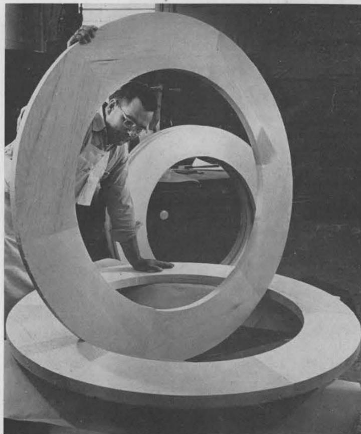
**GIANT RINGS** shown in this photo will be laminated together to form a single pattern. Richard B. Hicks checks grain structure and joint positions in the rings prior to the gluing operation.
